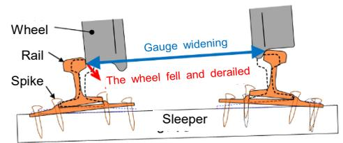
Image of a derailment caused by gauge widening
