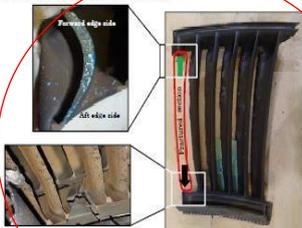
Taken from the direction of black arrow Red line: Fractured section of a stator vane (taken from the front side)
