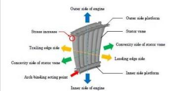
Arch-Binding refers to the condition of adjacent segments that are stuck tight, and the free movements of the adjacent segments are impeded.
