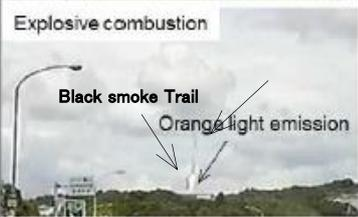
the left wing was broken → the fuel was discharged (ignited) → the right wing was broken → crashed
