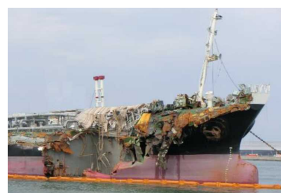
Oil tanker HOUNMARU after contact with a bridge
