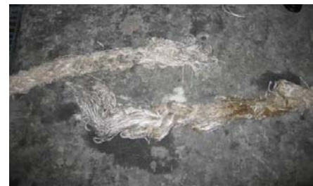
The Broken part of the Line
